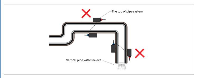
• For the open pipe or half full pipe, the transducers should be installed at the bottom of U pipe.
